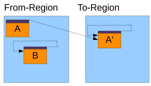
Writing an object in a From-Region will trigger an evacuation of that object to a To-Region and the write will occur in there.
